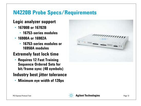
Here are the key specs for the N4220B probe.
