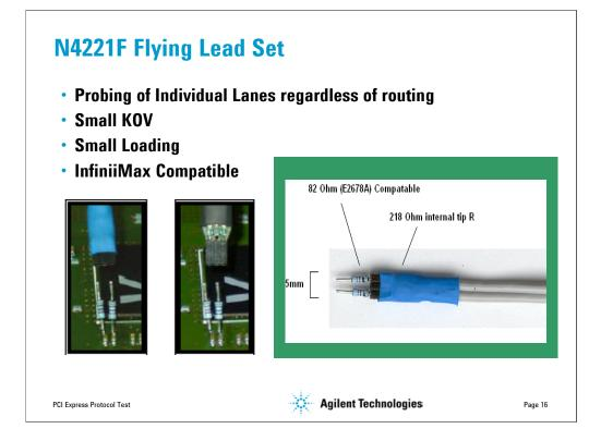
The flying leadset is ideal for customers who may have no board space for a midbus footprint, or who's midbus footprint may have accidentally disappeared between board revs. It provides full speed access to the 2.5Gb/s, and is small enough to probe in extremely tight spaces. It provides support for up to x16 PCI-E, and has the added benefit of being compatible with the Infiniimax scope probes as well (they both use the same 82-ohm resistors).
