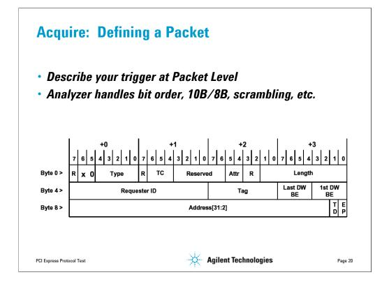
The N4220B allows you to define your packet header with great detail (up to 24bytes) for very precise triggering and searching. The N4220B also handles all of the bit ordering, scrambling, 8b/10b encoding, etc.
