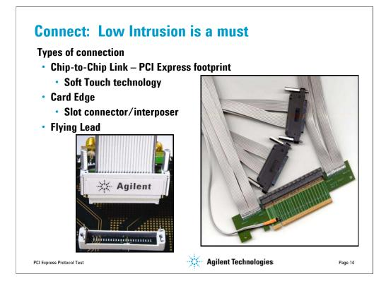
There are several types of connections that can be made to a PCI-E link. For chip-tochip links, there is a standard PCI-Express footprint that Agilent probes using our soft touch technology. For card edge applications, we offer what is commonly called an interposer, or sometimes called a slot connector. And for applications where there is no place to probe, we offer a flying lead probe that allows access to the 2.5Gb/s data.
