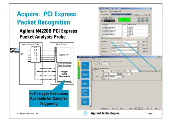
This gives you an idea of how the packet recognizers work. When you compare this to the slide three before this one, you can see how much easier it is to trigger on a complex packet, and how it does not consume the logic analyzer resources (which is especially important for the larger lane widths where a packet can start in multiple lanes and the trigger must look for it in each of those lanes). Each N4220B has four of the packet recognizers per direction built-in to it (for a total of 8).
