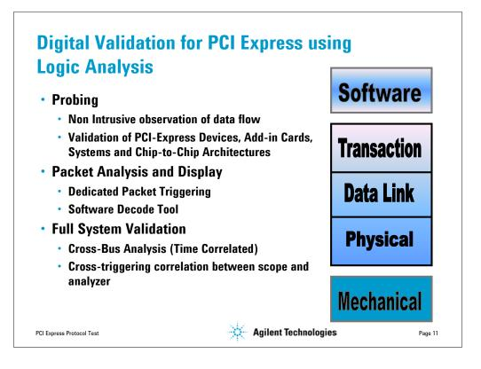
The Agilent logic analysis solution for PCI Express. Our packet analysis probe adds value when validating anywhere from the physical and transaction layers.
