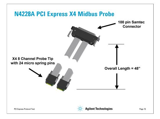
The N4228A is a half size midbus cable that is ideal for x1, x2 and x4 lane widths where board space is at a premium. It is the smallest probe available on the market today.
