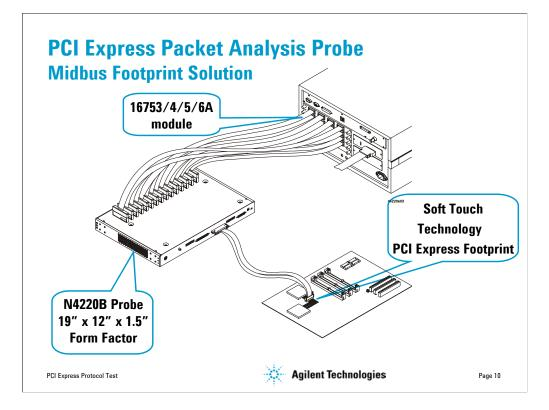
The general look of the solution will be probing the target system with 1 of 2 types of probes (Mid-bus, Slot Interposer), probe cables extend from the front of the Analysis Probe (a rack mount width, ~1 ft. deep by ~ 1.5 in. high "pizza" box). The 16754 family logic analyzer cables plug directly into the top of the Analysis Probe box along the back without needing an adapter.
