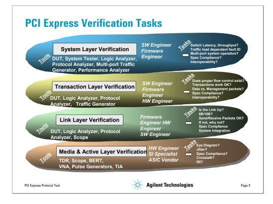
At each layer from the media/physical layer to the system layer, different tasks requiring different tools by engineers with different skill emphasis are required to ensure a properly functioning product.
