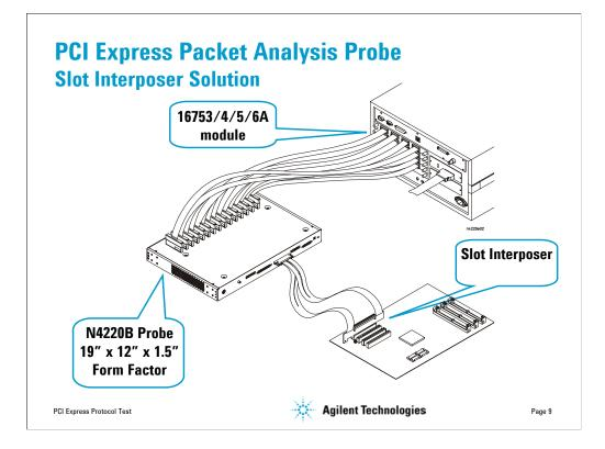
The general look of the logic analysis solution is probing the target system with 1 of 2 types of probes (Mid-bus, Slot Interposer), probe cables extend from the front of the Analysis Probe (a rack mount width, ~1 ft. deep by ~ 1.5 in. high "pizza" box). The 16753 family logic analyzer cables plug directly into the top of the Analysis Probe box along the back without needing an adapter.
